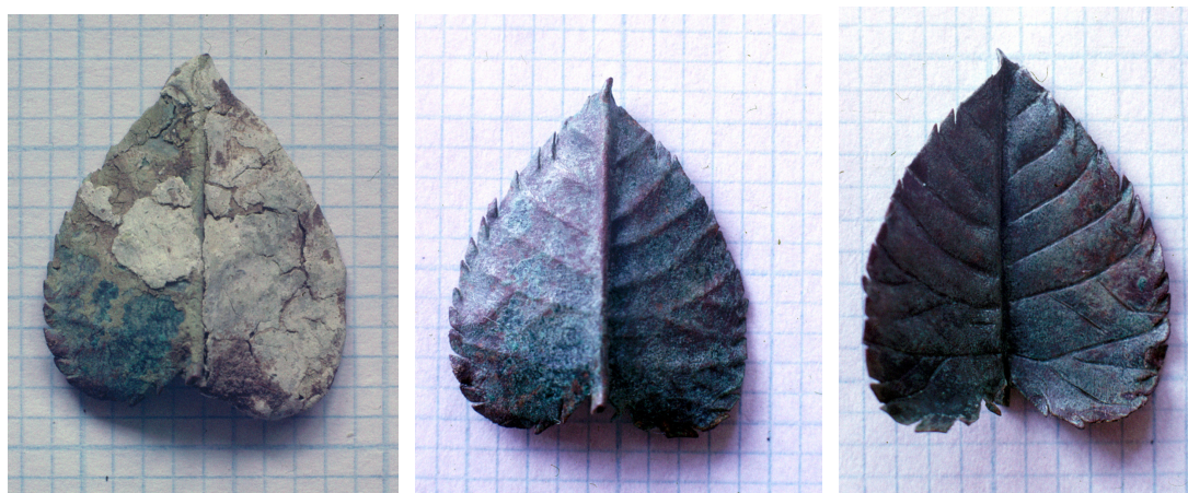
Figure 94. The copper leaf, as found partly covered with limescale and the two sides after cleaning. The graph paper has 2mm squares.
