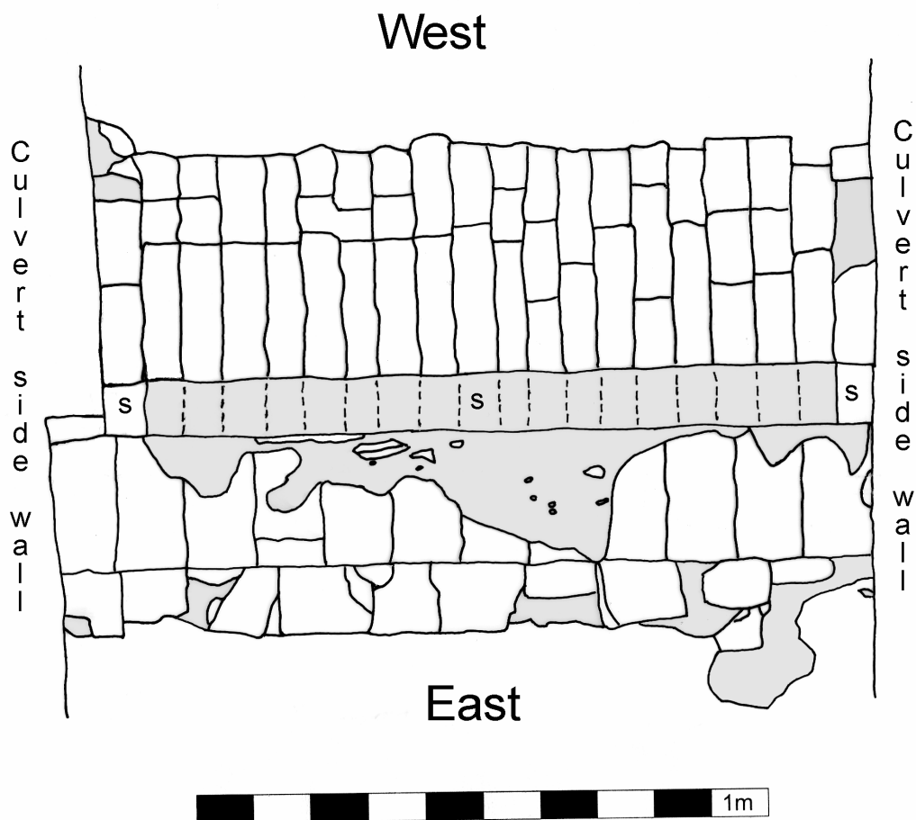
Figure 81. Plan of the slot in the floor at the beginning of culvert section 1. S S S = slot. Grey = mortar.
