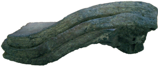
A stack of roof tiles fused together and warped, found in the Whitehall garden excavation
