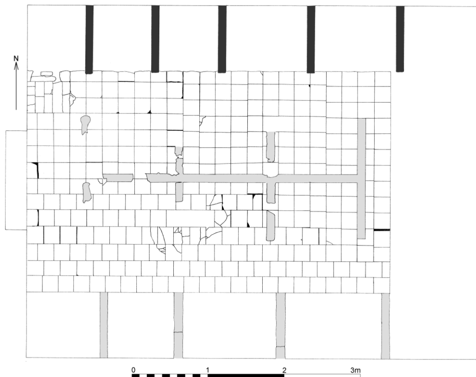
Figure 55. Plan of the floor of cellar 7 showing the bottom of the wine racks (dark grey) and the scars from the demolished ones (light grey). The blank areas around the edge of the cellar are brick-floored.
