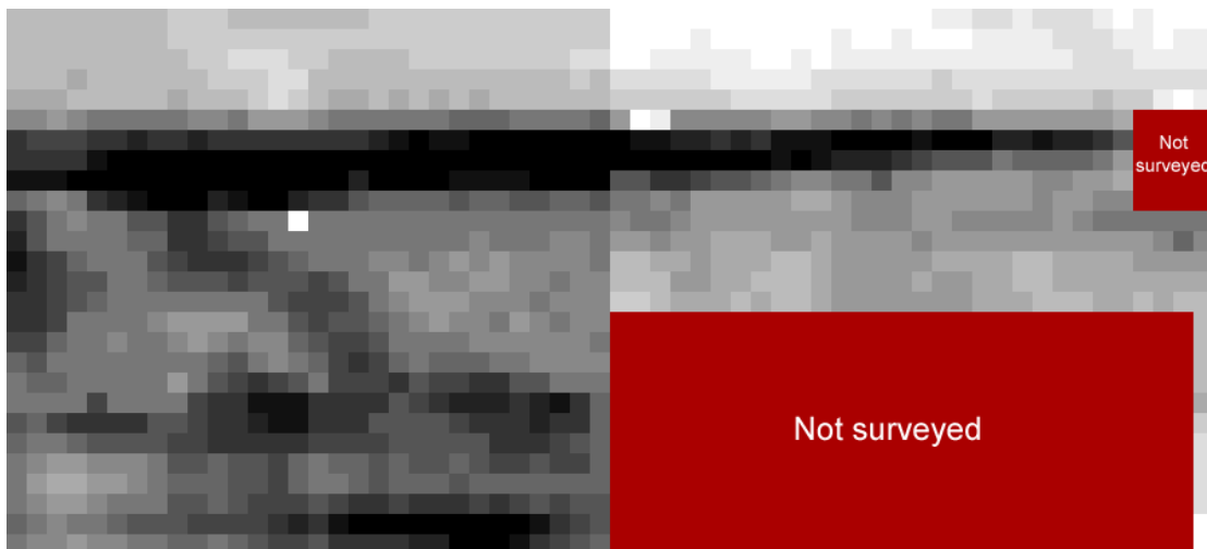
Figure 24. Resistivity survey on the site of the pond created during the floor alleviation work. Scale: one square per metre. North at the top.
