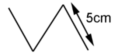
Figure 33. Corner 6. The carpenter's mark on the north side of the main tie-beam
