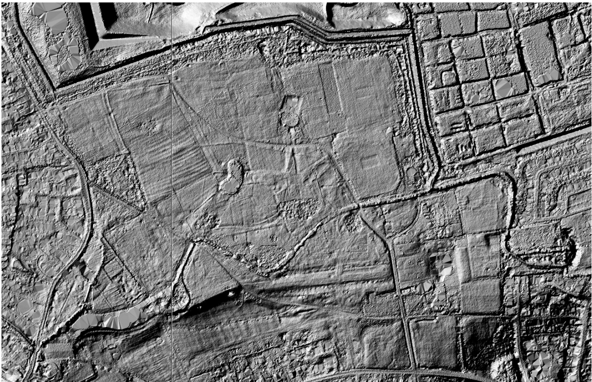
Figure 19. Lidar scan of the park. Azimuth 120, height 35.
