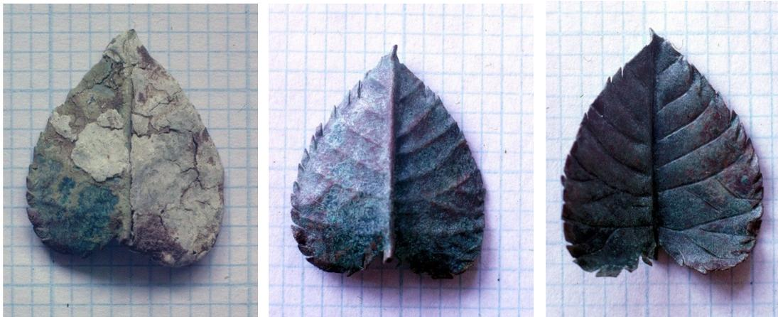
Figure 180. The copper leaf, as found partly covered with limescale and the two sides after cleaning. The graph paper has 2mm squares.
